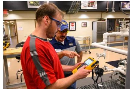
Cleveland observes student MGCCC William Mansfield use a Fluke 754 Document Process Calibrator to communicate through HART with a Rosemount pressure transmitter.
